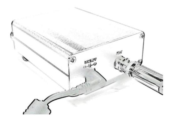
Connect the Antenna to FM Transmitter.
